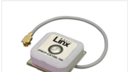
TE 产品编号ANT-GNCP-CA158L160 Antenna GNSS L1 15x15 LNA 1.13 UFL
