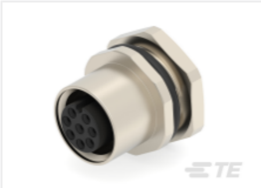
TE 产品编号T4133012081-000 M12,FRONT MOUNT,FEMALE,A,8P, SOLDER WIRE
