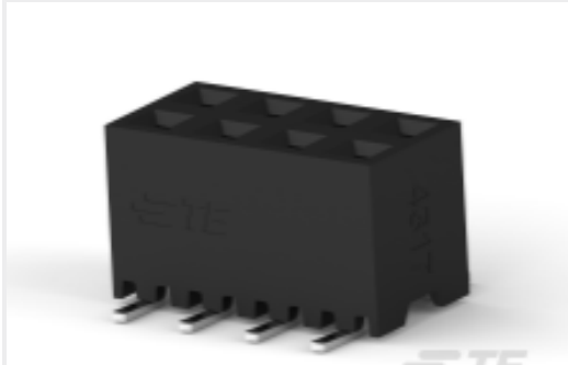
TE 产品编号2314844-8 8P,2MM,B-B,REC,DRVT,SMD,0.1AU, TB,W/CP
