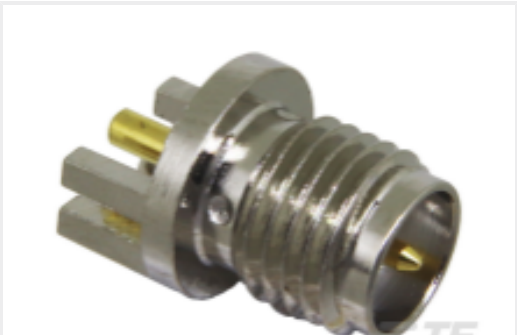
TE 产品编号L9000248-01 RP-SMA Jack 50 Ohm .031 PCB Edge Mount
