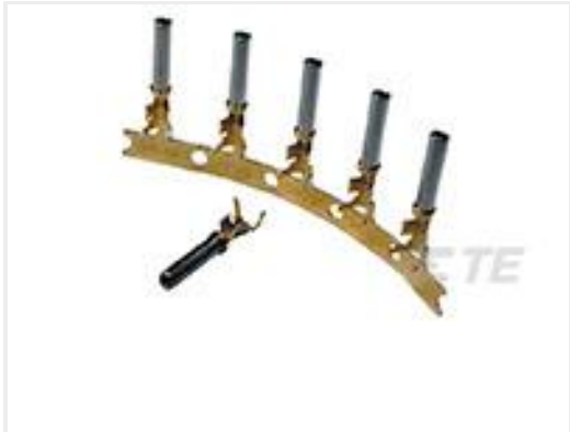
TE 产品编号1062-14-0144 SOC, SF, SIZE 16, 14-18, AU/SN
