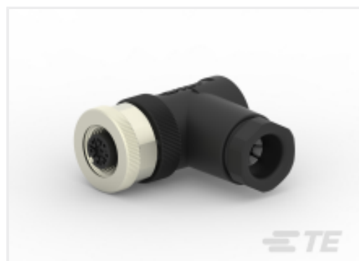
TE 产品编号T4112002081-000 M12,FEMALE,RA,A CODE,8P,PG9, GOLD
