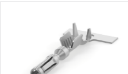
TE 产品编号770520-6 AMPSEAL,TERMINAL,TIN PLATE,22-24AWG WIRE
