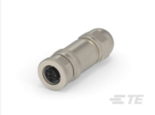
TE 产品编号T4110011021-000 M12 F, 2P GOLD A_CODE S SHIELDED PG7
