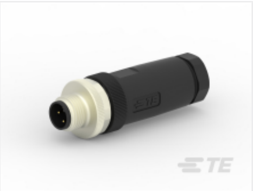
TE 产品编号T4111002041-000 M12,MALE,STRAIGHT,A CODE,4P, PG9,GOLD
