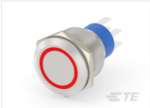
TE 产品编号6-2213772-7 AV22 DPL 3A MOVE RING LED RED 24V
