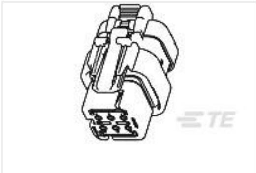
TE 产品编号776531-3 AS16,PLUG ASSY,ST,06P,E SEAL, CODE C
