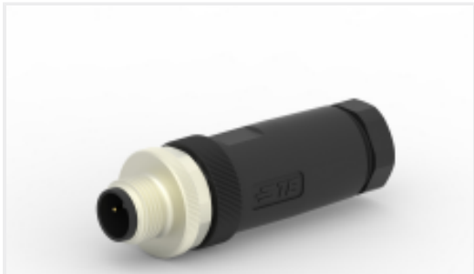
TE 产品编号T4111002021-000 M12,MALE,STRAIGHT,A CODE,2P, PG9,GOLD
