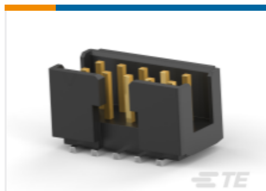
TE 产品编号1-2373376-0 10P,2MM,SHRD HDR,DRV,T,SMD,0.1 AU,TB
