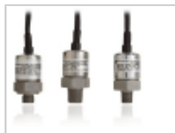
2500 PSI, 1/4MNPT, 20 mV/V, 2ft 4 wire C
