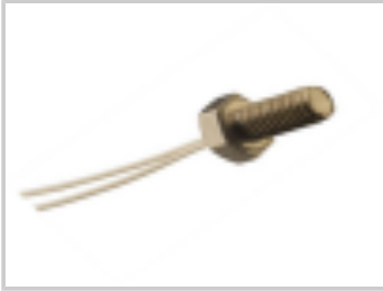
Probe, M5 Hex Nut, 5K +/- 0.2'C, 200mm
