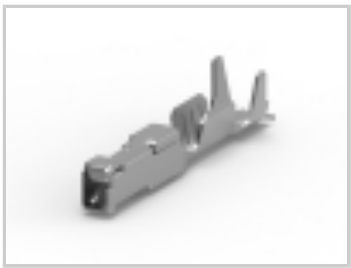
Contact,female0.64, 18AWG, CuNiSi, Sn
