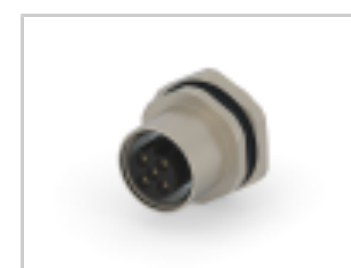
M12, FRONT MOUNTING, FEMALE, B, 5P, 0.2M WIRE
