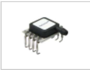
HCEM050DUE8P5; PRES; 0...50m,bar; 4V; 5V
