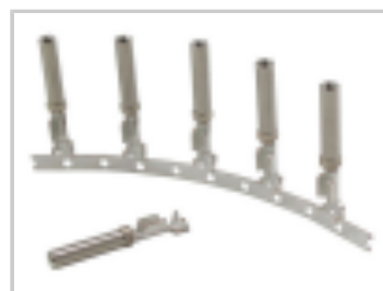
SOC, SF, SIZE 16, 18-20 AWG, NI/SN
