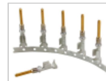
PIN, SF, SIZE 16, 14-18 AWG, AU/SN
