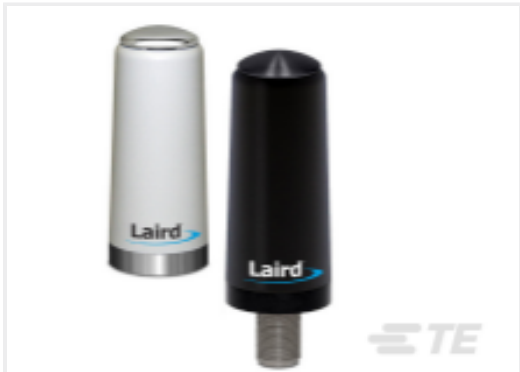
TE 产品编号TRA6927M3PW-001 OMNI,DB,Ph,698/1710 MHz WHT,3 dBi,100W,
