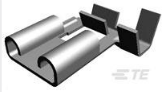
TE 产品编号62718-2 250 FASTON FLAG REC 22-18 AWG TPBR
