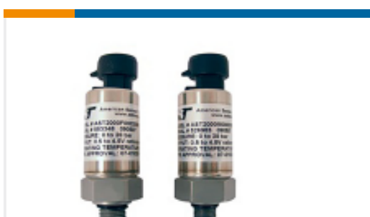
TE 产品编号11100565-00 20 BAR, 3/8-24UNF Male, 0.5-4.5V, Packar
