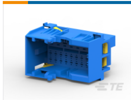
TE 产品编号1-2112890-3 25POS, MIXED,TAB HSG,ASSY
