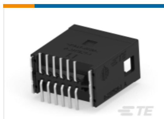
TE 产品编号2317527-1 2X6POS,NANOMQS,HDR ASSY, 180DEG,SMD,COD A
