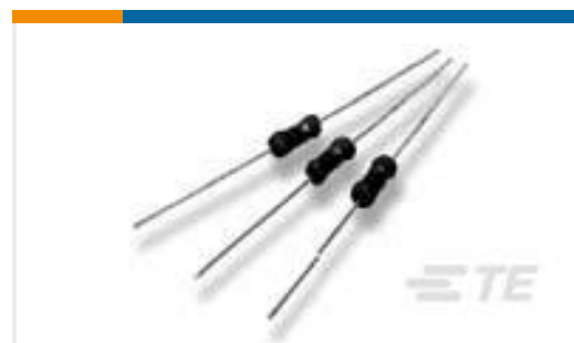
TE 产品编号1-1625890-1 2W SM M/OX 5% 150K
