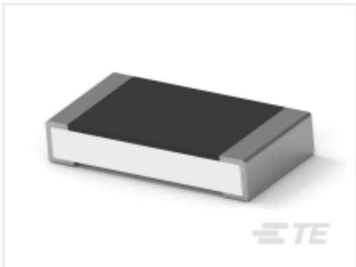
TE 产品编号5-2176389-6 RQ 1206 402R 0.1% 10PPM 5K RL
