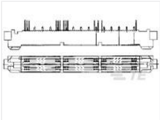
TE 产品编号5767032-3 MICT,788PLUG,114,ASSY,.025,REC BAG
