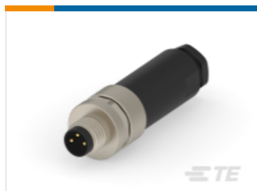
TE 产品编号T4011008031-000 M8,SCREW, MALE,S,UNSHIELD,3P, GOLD
