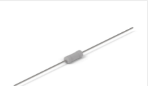
TE 产品编号7-1676123-9 1/2W SM M/OX 5% 1K5
