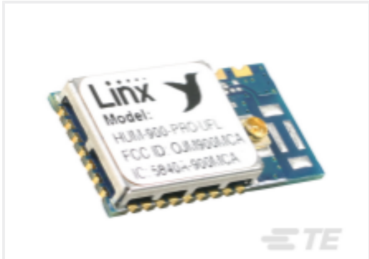
TE 产品编号HUM-900-PRO-UFL Module HUM-PRO 900MHz FHSS FM XCVR FCC
