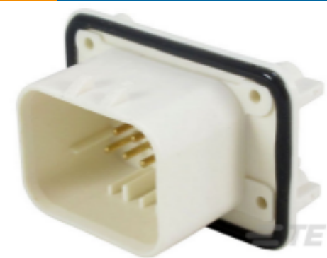
TE 产品编号 1-776267-2 14POS, PIN DIA 1.3, HDR ASSY, 90DEG, COD 2
