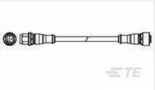
TE 产品编号1-2273112-4 M12 strgt plug to M12 strgt socket AA
