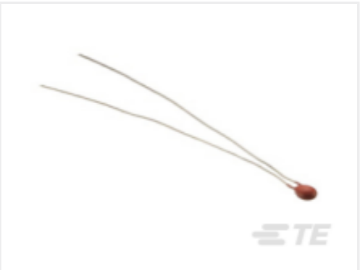
TE 产品编号GA50K6A1ID DISCRETE 50K OHMS,+/-1.0C FROM 0C TO 70C
