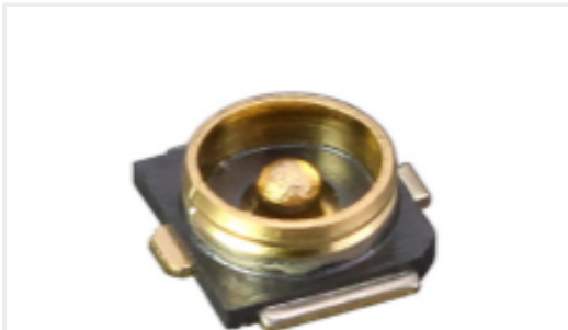
TE 产品编号CONMHF4-SMD-G-T MHF4 Jack 50 Ohm PCB Surface Mount
