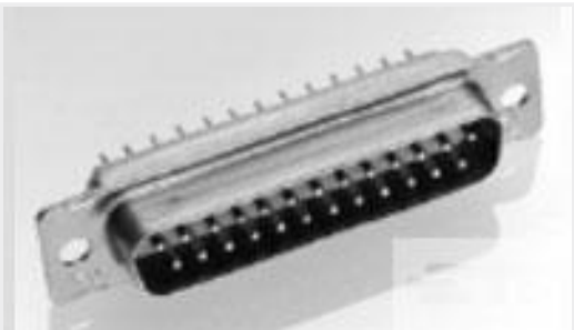
TE 产品编号205166-1 AMPLIMITE,ASY,PLUG,STD,109,3
