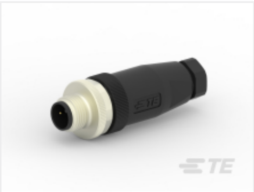
TE 产品编号T4111001021-000 M12,MALE,STRAIGHT,A CODE,2P, PG7,GOLD
