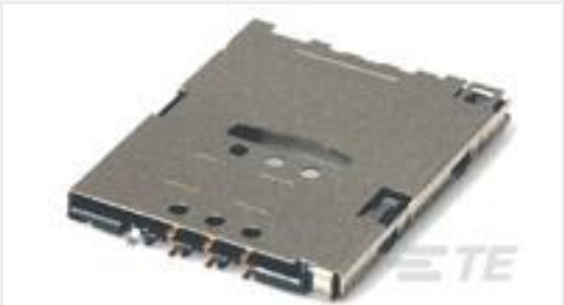
TE 产品编号1981959-1 PUSH PUSH SIM H1.87 SWITCH EMBOSS ASSY
