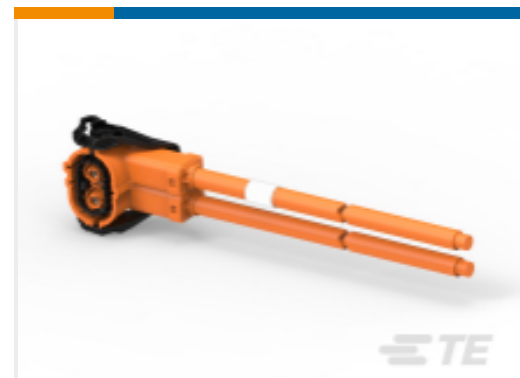
TE 产品编号1-2286946-4 2POS,HVP800,90 DEG,35 SQMM,COD A
