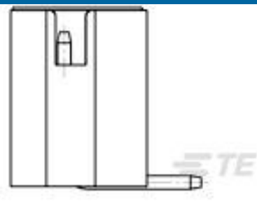
TE 产品编号1775470-2 HPI CONN., 2.0MM, V/T, SMT, 2P, 80U"
