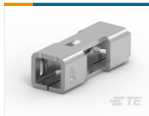
TE 产品编号2834171-3 ULTRAMINIATURE SLIM CONTACT
