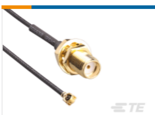
TE 产品编号CSH-SGFB-200-UFFR SMA to U.FL/MHF1 200mm 1.32 OD
