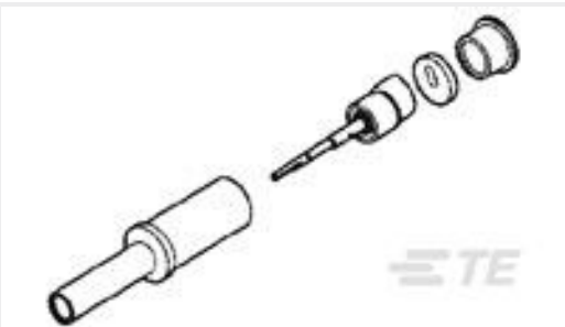
TE 产品编号1757624-1 SZ 8 COAX PIN,RG142,HEX CRIMP
