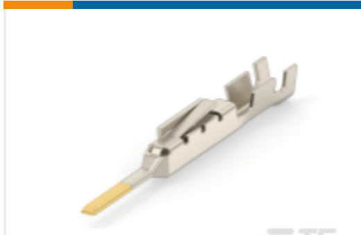
TE 产品编号1318108-1 Contact: Component To Wire ; 5A, 28-18 wire size, gold plated
