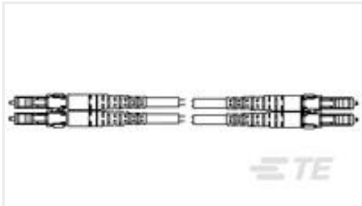
TE 产品编号8-2061348-1 FOSM LEAD LC/DPX ODVA - LC/DPX 120M
