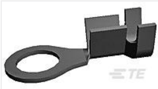
TE 产品编号40661 RING 190(4.82 MM) TERMINAL 18-14 AWG BR
