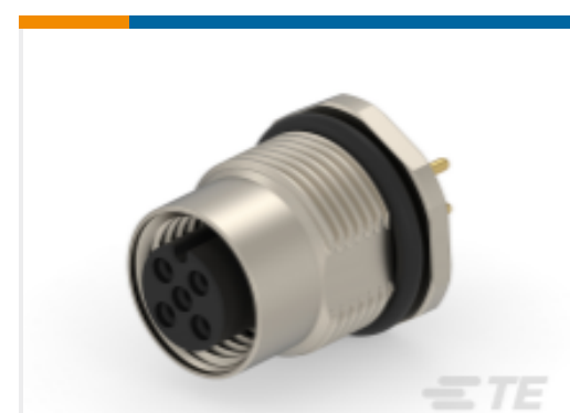
TE 产品编号T4141042041-000 M12,REAR MOUNTING,FEMALE,A CODE,4P
