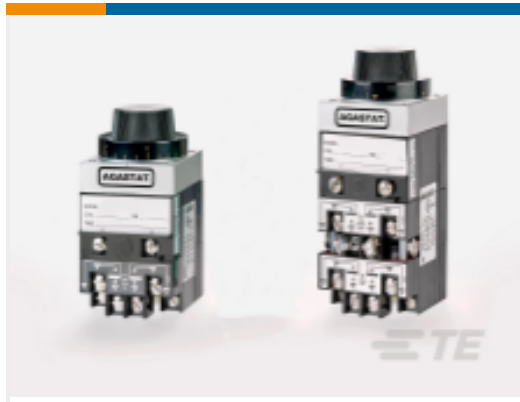
TE 产品编号5-1472973-5 7012NH=RLY,STD,ON,2P,48VDC, 30MIN
