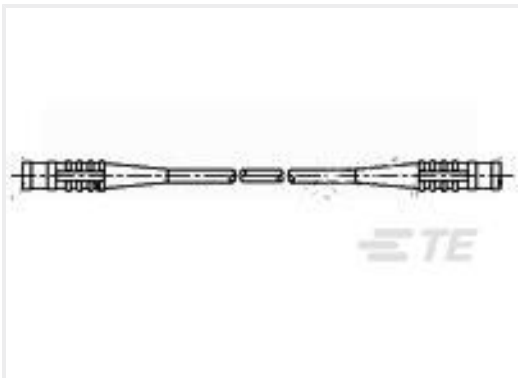
TE 产品编号1337814-2 50 OHM COAX SMB STR PLUG STR P COMPLETE
