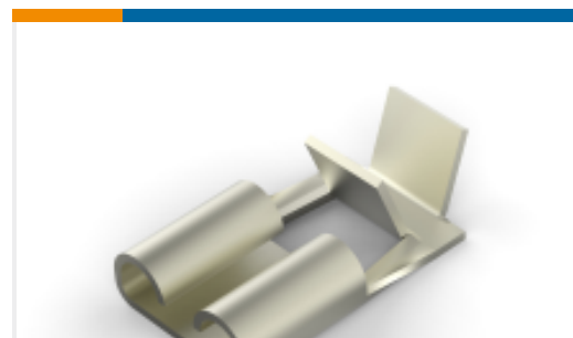
TE 产品编号1217972-2 250 FASTON, FLAG, REC., 18-14 AWG, NPST
