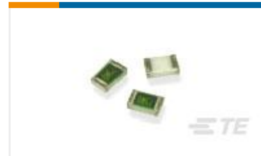
TE 产品编号3-2176093-9 RP 2A 0.25W 23K7 0.1% 25PPM 1K RL
